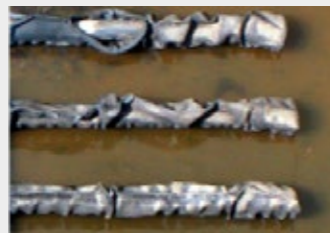
Fig. 2: Destroyed by chemical reaction with oil
